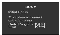
Press on the remote control or on the TV front panel to start Auto Program, or press to exit.
