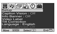
Select closed captioning options, display the name of the currect program and its remaining time, label video inputs, adjust tilt correction (available only for KV-24FS120), select menu languages, or run a demo of the menus.
