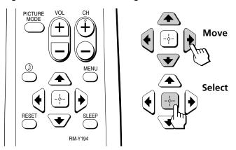
To navigate on the on-screen menus, use the "arrow" buttons ( $\spadesuit$ ,  $\clubsuit$ ,  $\spadesuit$ ) to move the cursor. Pressing these arrows will cause the cursor to move in the corresponding direction. Pressing center button  $\oplus$  will allow you to select an option.
